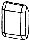
Fig. 129. A ten-sided prism, with two broad faces, terminated by two principal planes, corresponding with the lateral planes.
